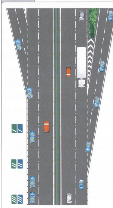
**Purpose:** Slip roads provide you with entry and exit points to a motorway or dual carriageway. These normally join the main carriageway from the left.
